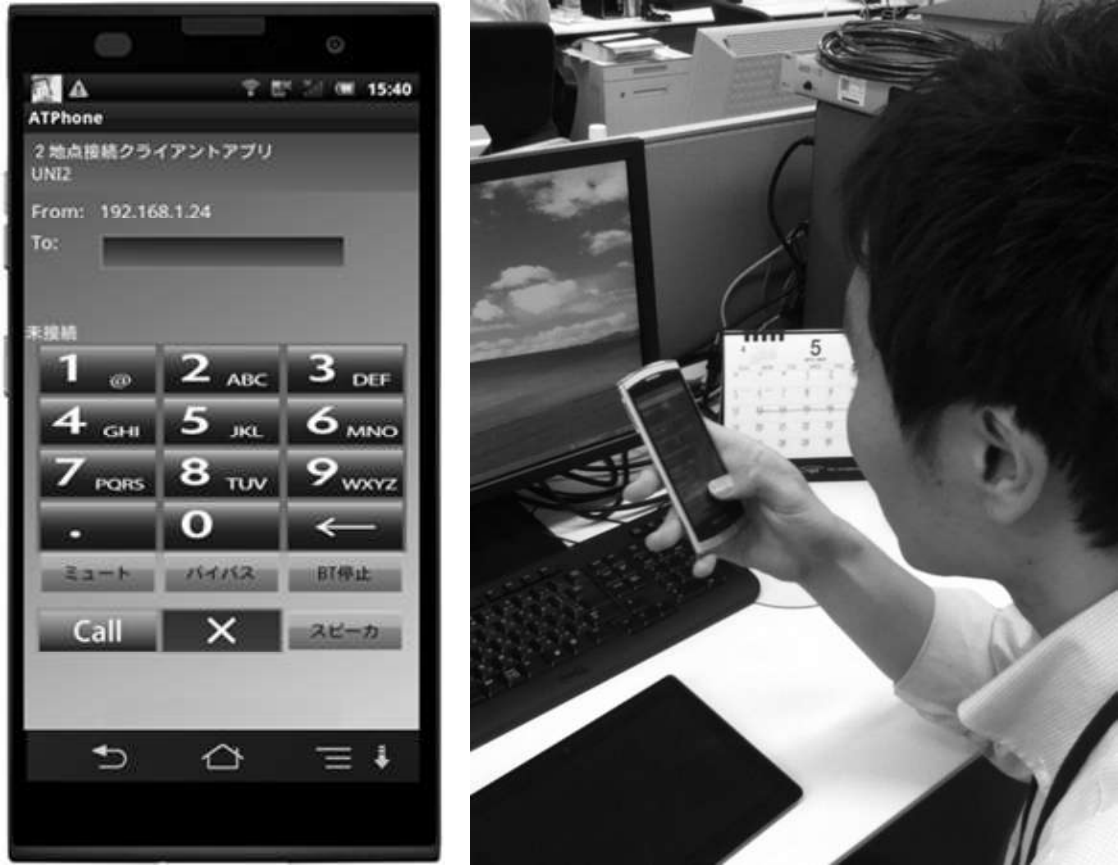
Figure 6.3. Photograph of VoIP phone prototype equipped with proposed AEC method.
