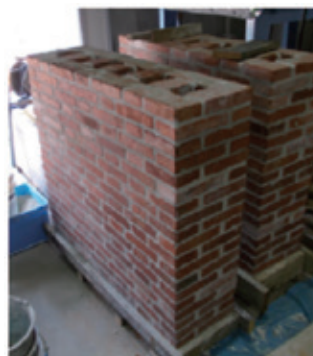
Photo 1 Specimen Sample of Brick Wall
