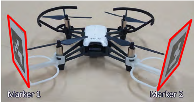
Figure 4.1: DJI Tello used in the first implementation mounted with two AR markers.
