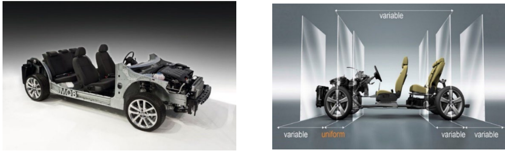
Figure 2-7: Volkswagen's MQB Platform (Source: Volkswagen AG)
