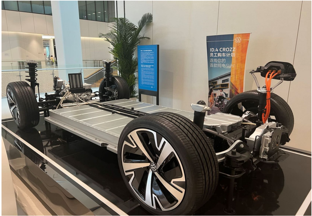
Figure 2-8: VW's MEB Based Chassis with Battery Pack (Source: shot by author)
