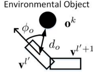
Figure 4.5. Compute the relative posture of a robot link with an interacted object in environment.
