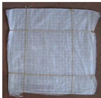
Fig. 3-2-2. Non-woven fabric wrapped around a wire mesh frame as a biomass carrier.
