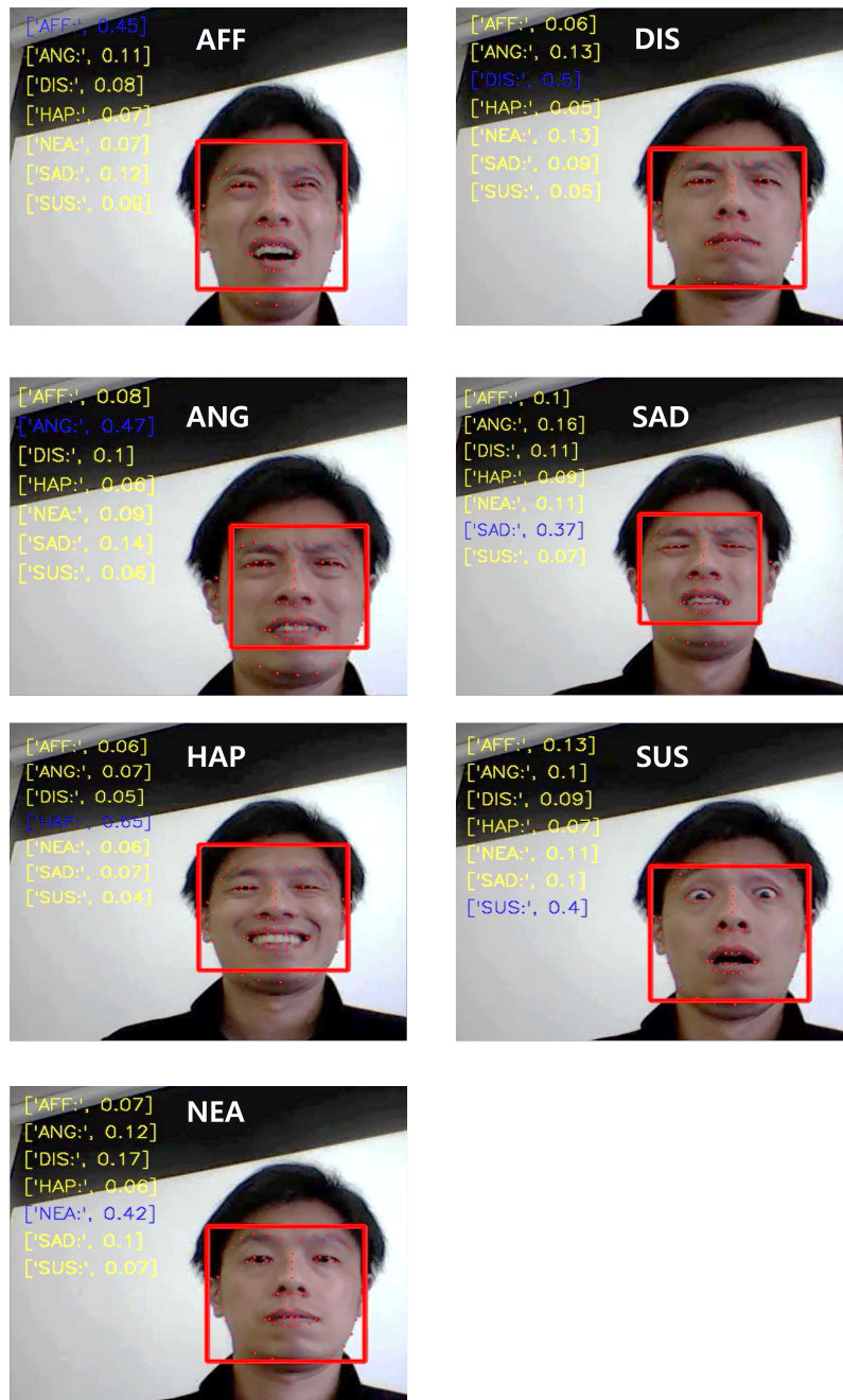
Figure 5.16. Testing of the user's emotional intensity (ID: 40AS06) in real-time. Blue text indicates the highest intensity. AFF, ANG, DIS, HAP, NEA, SAD, and SUS means the fear (afraid), angry, disgust, happy, neutral, sad, and surprise expression.
