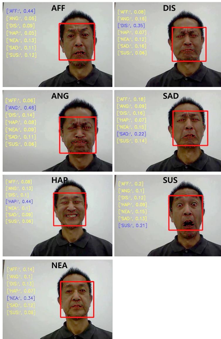
Figure 5.14. Testing of the user's emotional intensity (ID: 60AS28) in real-time. Blue text indicates the highest intensity. AFF, ANG, DIS, HAP, NEA, SAD, and SUS indicate the fear (afraid), angry, disgust, happy, neutral, sad, and surprise expression.
