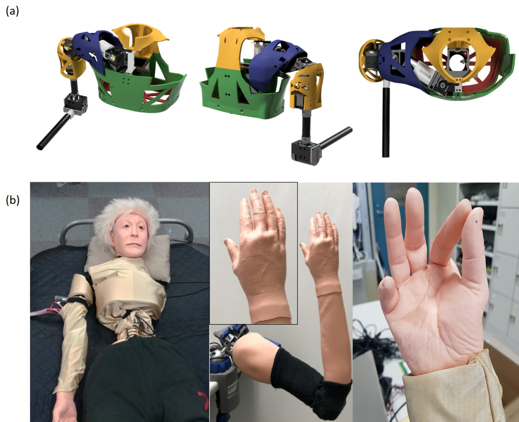
Figure 3.6. Pictures of exterior design of the patient robot with artificial skin (a) Shoulder complex (b) Elbow complex.
