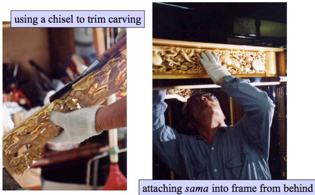
Kumi photo 31: trimming and attaching transom carving ( sama )
