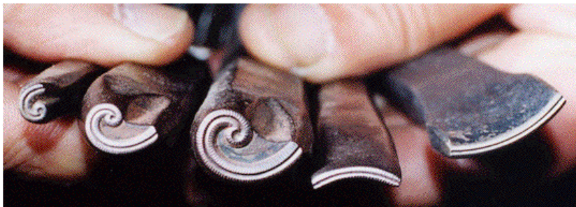
double edged whole pattern burins ( moyou tagane ) for making arabesque designs
