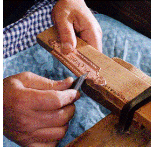
he is smoothing the edge with a knife by holding it tightly to the metal and sliding it along
