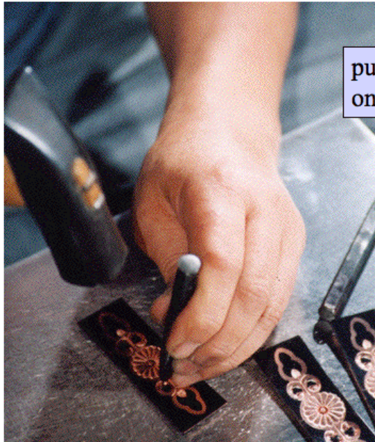
Kan photo 61: punching the design on cut out ( sukashibori ) kanagu
