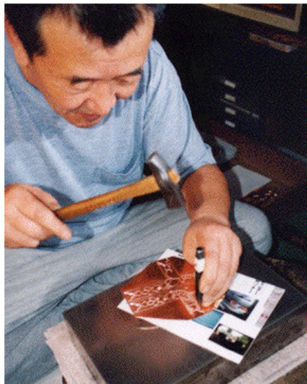
Kan photo 36: hitting the tagane with metal hammer
