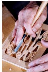
working on wakizama using uchimaru nomi ( gantou ) (see Cho photo 26) borders left on for support
