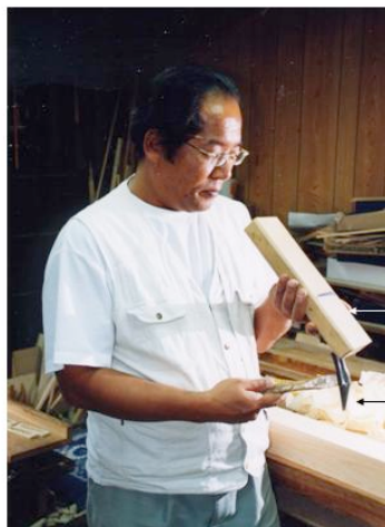
Kiji photo 08: Tsuji Toshimasa adjusting the plane blade
