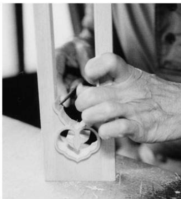
Kiji photo 14: final shaping of drawer decoration – complex pattern
