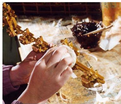
rubbing with mawata to press and smooth the leaf and remove overlaps
