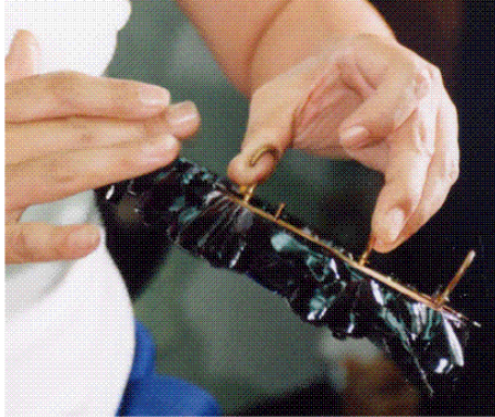
Junji holding hooks at the back of the carving and tapping to remove excess bengara urushi
