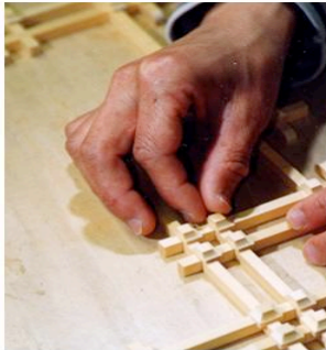
Kuuden photo 31: attaching komasu to the beams with rice glue
