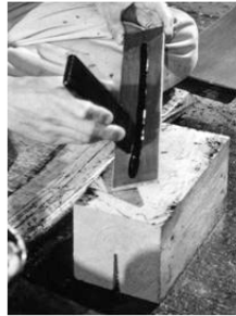
with a brush, nakanuri urushi is applied by making a streak down the middle of the board
