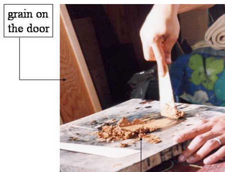
Nuri photo 13: mixing tonoko with water (2 nd stage of making kataji )
