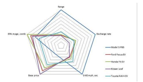
The Model S has significant advantages in Range, Recharge rate, and 0-60 acceleration over competing EVs- although this performance comes at a much higher price. <u>Image source</u>: Reynolds, 2012
