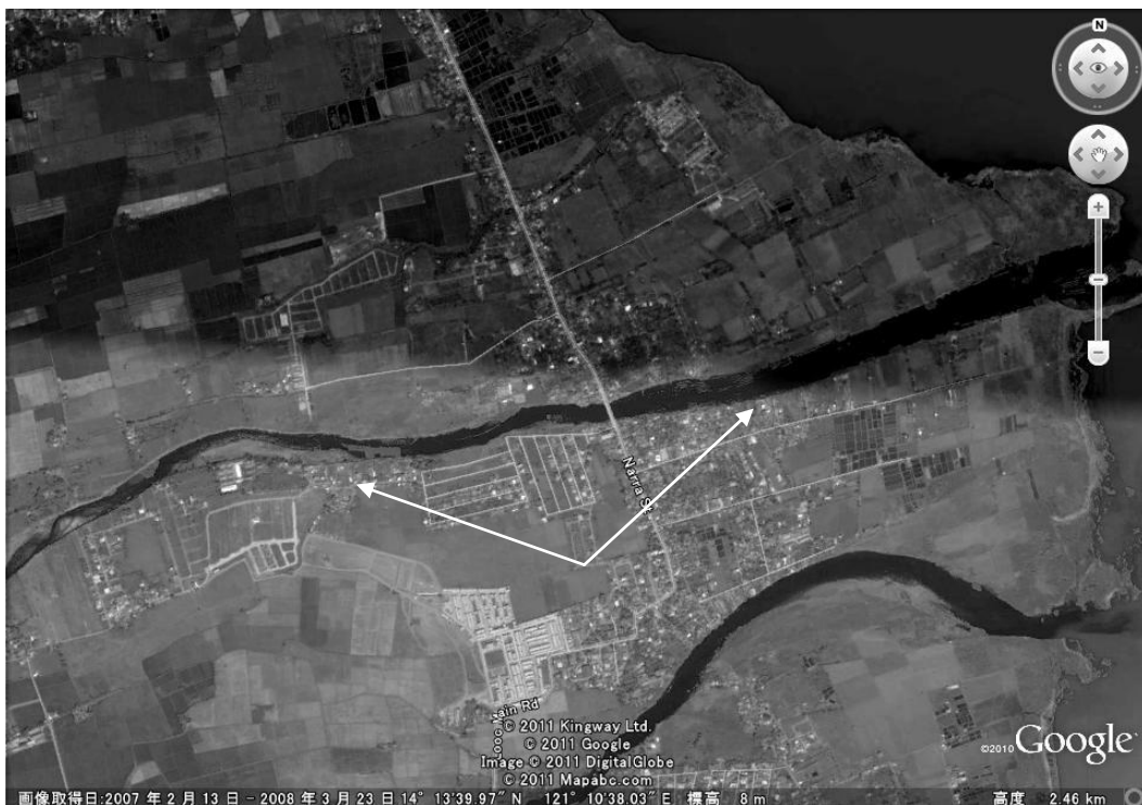
Figure 6.21: Alteration of the buffer zones along the lower reach of the San Cristobal peri-urban sprawls. The vegetated in channel deposition (arrows) reflect the loss of stream competency and
