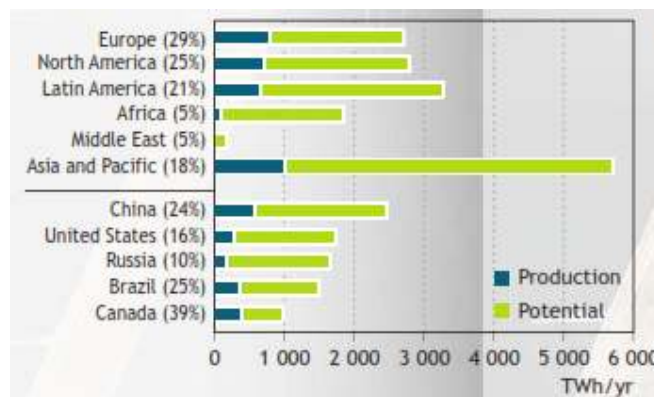
Figure 2.1 The ratios of potential and production of hydro power in the world.
