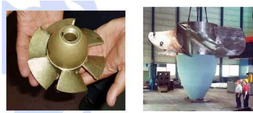
Figure 2.16 The cast bronze propeller turbine (a) designed at Kathmandu University (b) Andritz
