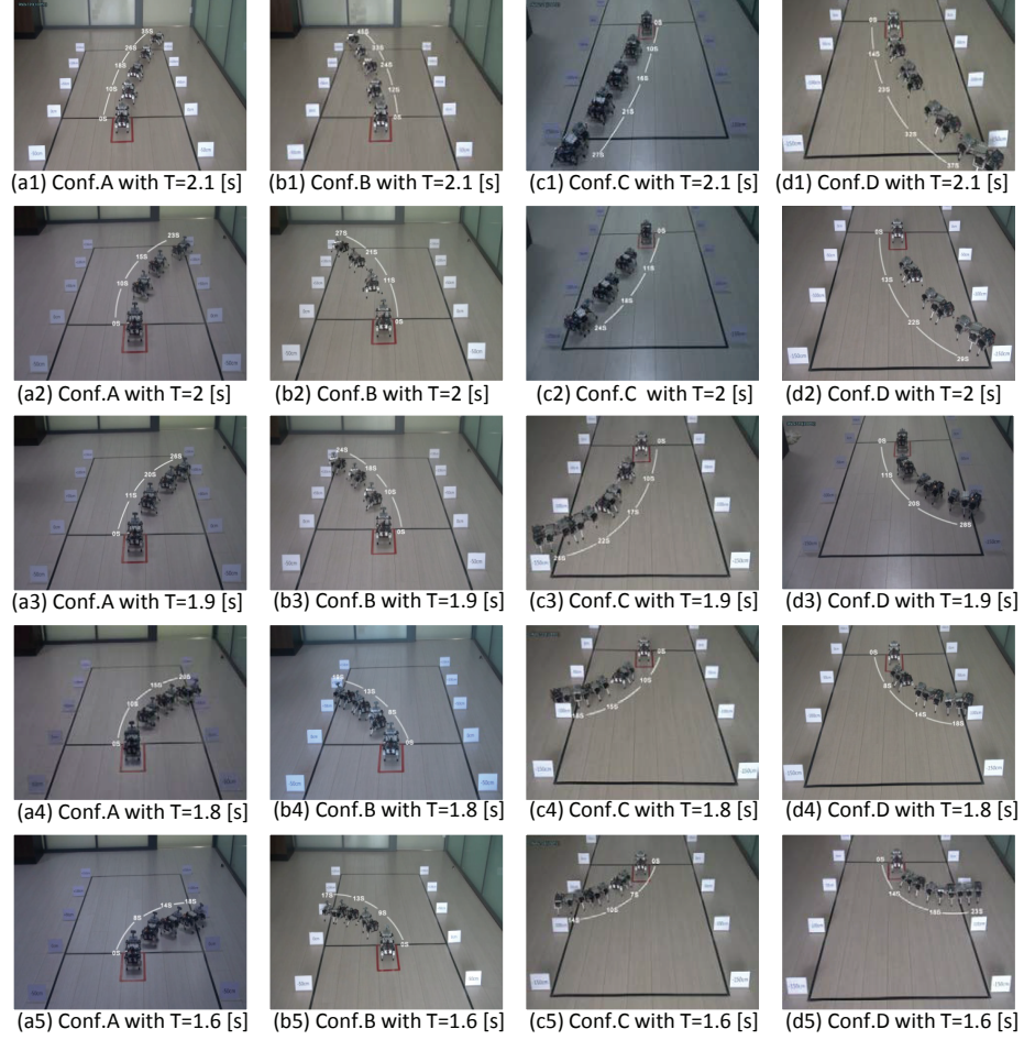
Figure 6.5. Position tracking for turning gaits of standard configuration transitions A, B, C, and D with different speeds. (a1) Configuration A with T = 2.1 [s], (a2) Configuration A with T = 2 [s], (a3) Configuration A with T = 1.9 [s], (a4) Configuration A with T = 1.8 [s], (a5) Configuration A with T = 1.6 [s], (b1) Configuration B with T = 2.1 [s], (b2) Configuration B with T = 2 [s], (b3) Configuration B with T = 1.9 [s], (b4) Configuration B with T = 1.8 [s], (b5) Configuration B with T = 1.6 [s], (c1) Configuration C with T = 2.1 [s], (c2) Configuration C with T = 2 [s], (c3) Configuration C with T = 1.9 [s], (c4) Configuration C with T = 1.8 [s], (c5) Configuration C with T = 1.6 [s], (d1) Configuration D with T = 2.1 [s], (d2) Configuration D with T = 2 [s], (d3) Configuration D with T = 1.9 [s], (d4) Configuration D with T = 1.8 [s], and (d5) Configuration D with T = 1.6 [s].
