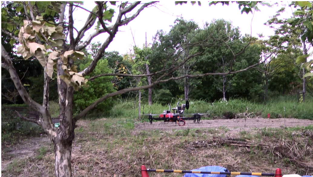
Figure 5.7: Aerial pruning robot flying with all the control components embedded on the hexarotor helicopter.
