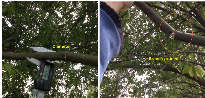
Figure 6.6: Diameter of the tree branch pruned in this experiment. Notice that in the right side picture is shown the cut produced by the circular saw.
