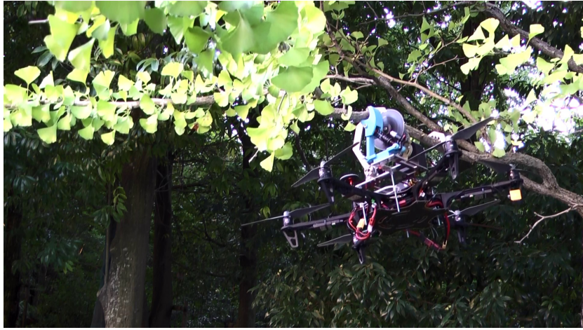
Figure 6.7: Sabertooth motor driver approach using the super helping hand to provide support at the moment of pruning.
