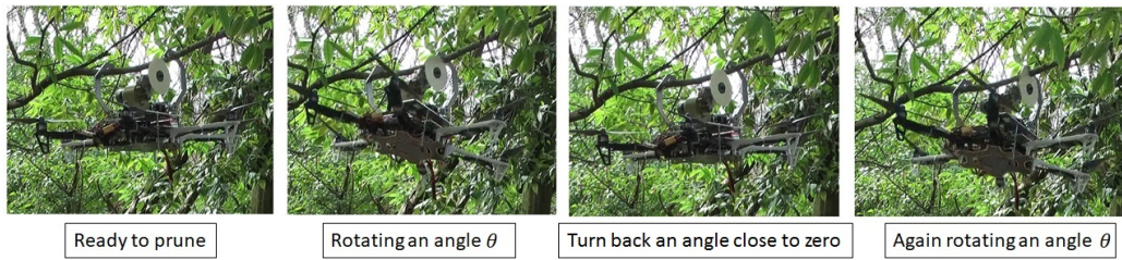
Figure 6.4: Real pruning sequence. From the left to the right, the pruning mechanism is idle and later, it starts pruning swinging repeatedly
