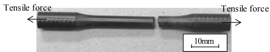
(a) Typical tensile fracture ( \phi 4 tension, 0.5v_f )
