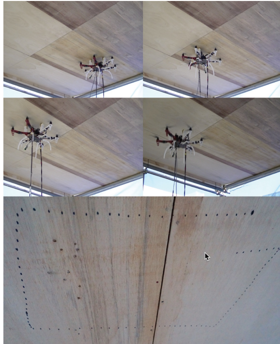
Figure 7.12: (Up) Video sequence showing the use of an industrial print head on the ceiling. The result can be seen in the lower picture.
