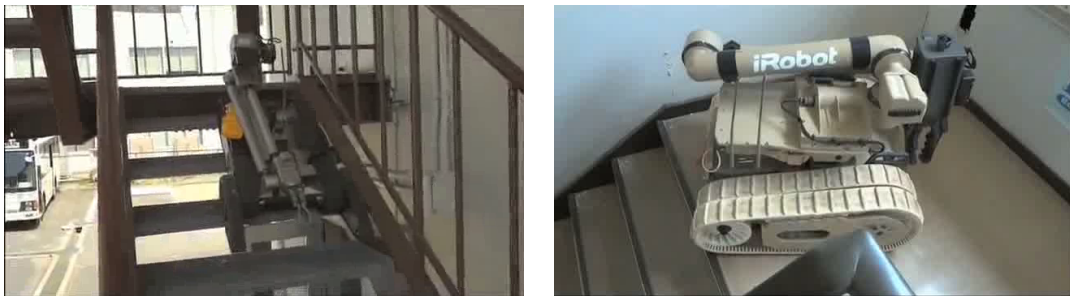
Figure 2.8: Photo of iRobot Packbot (left) and Warrior (right) during training exercises for a deployment in the destroyed Fukushima Daiichi power plant. Although specifically developed for use in a military environment, they were the first robots deployed in the Fukushima Daiichi reconnaissance efforts. (images taken from [2])
