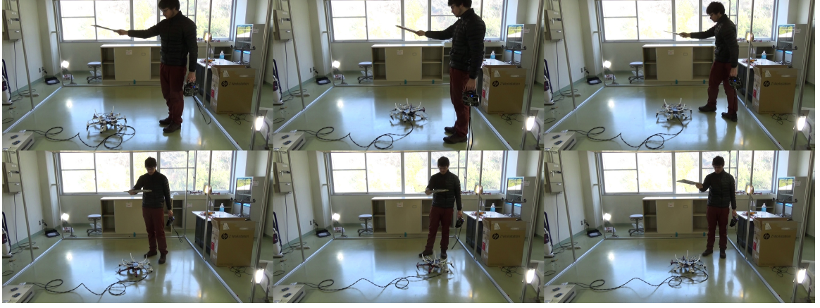
Figure 7.2: Video-sequence of testing of the dual camera system mounted on the hexrotor with a visual servoing task. The system successfully follows the marker held above it and correctly centers directly under the marker, even if it's held at an angle. ( https://youtu.be/Rp3i9mW-yBE )
