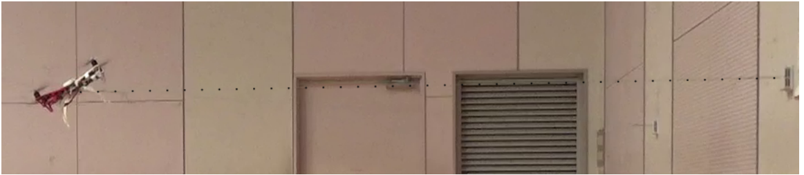
Figure 3.3: Photo of a test flight of the rope-based refined control prototype. In this test flight, the ropes were non-retractable. The position of the rope was marked with dots by hand to make them better visible.
