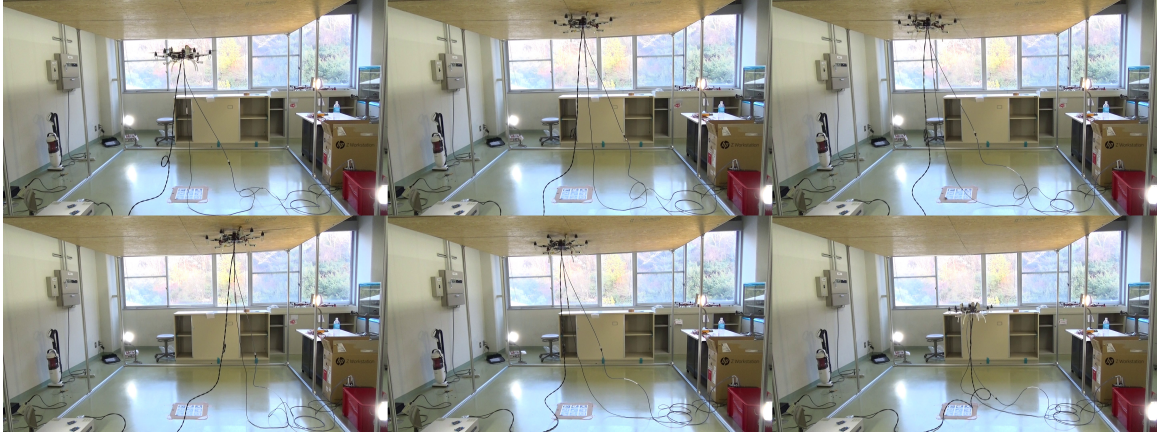
Figure 7.3: Video-sequence of testing ceiling engage, manual movement and disengage with paint marking payload. ( https://youtu.be/BVQZBh6Zw04 )
