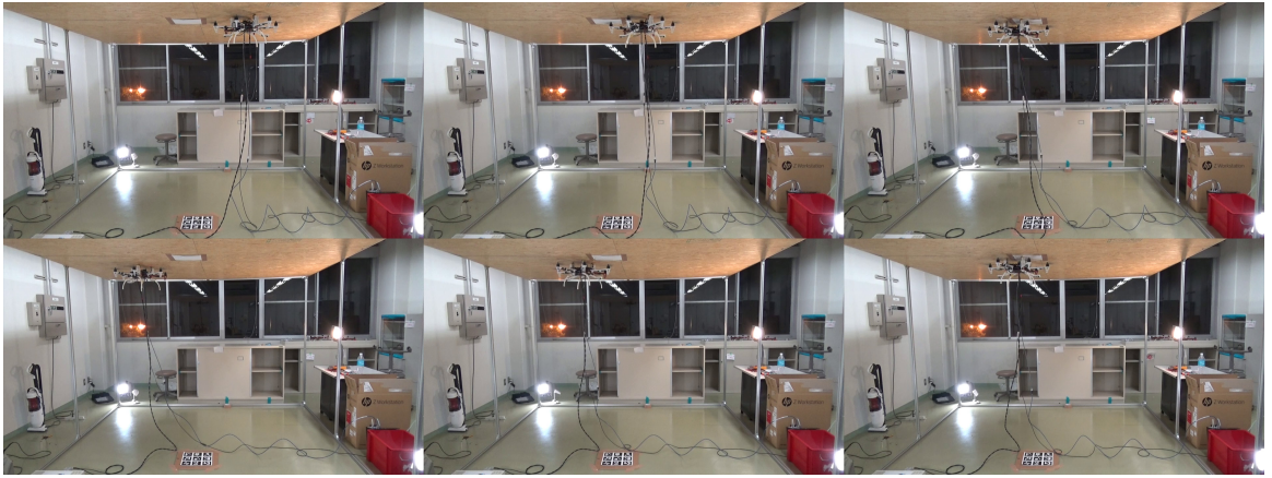
Figure 7.4: Video-sequence of testing the autonomous tracking of a target on the ceiling. ( https://youtu.be/FwOYFaVgGUI )
