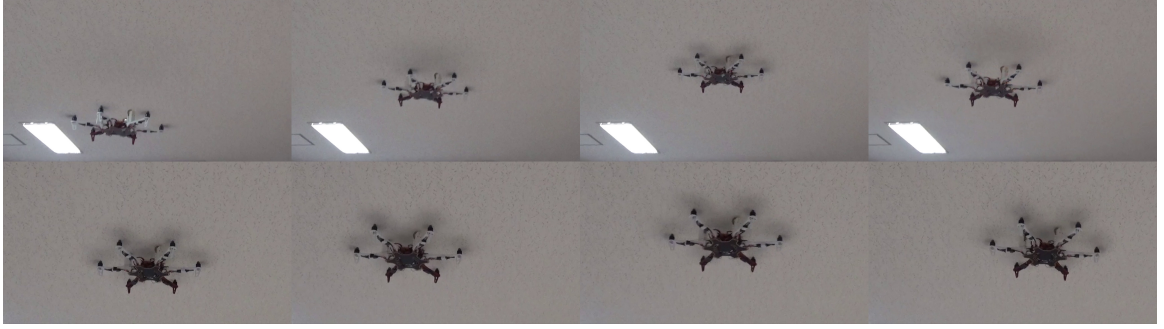
Figure 7.1: Video-sequence of an early ceiling docking, driving and disengage test. The test was performed on a 3m high ceiling. In the upper row, ceiling engage and disengage is shown. In the lower row, an open loop drive sequence driven by the Atmega micro controller on board is tested, where the system drives in a 30cm diameter circle. ( https://youtu.be/gEDIJqR9pS8 )
