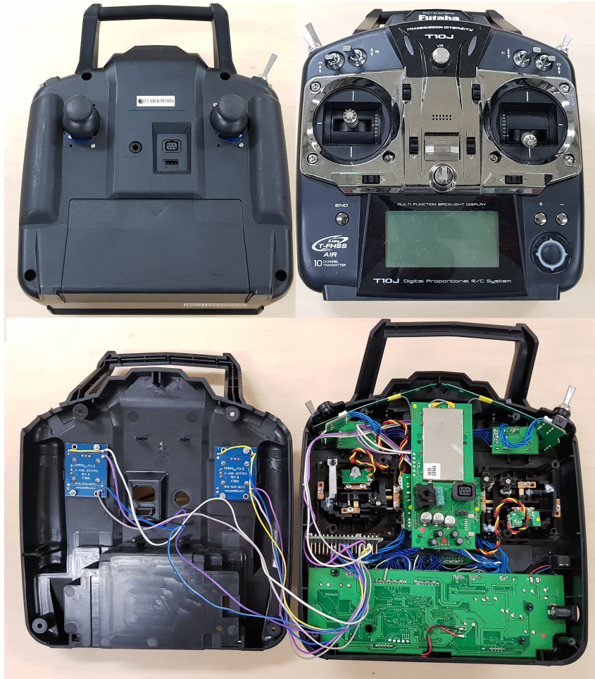
Figure 5.13: The custom remote used by the operator. Since generally radio remotes come with a maximum of four analog channels, we added two joysticks and a micro controller to the remote, making the simultaneous control of a total of eight analog channels possible.
