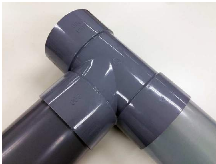
図 6.6: A T-branch for the experiment of the three modular pipe inspection robot
