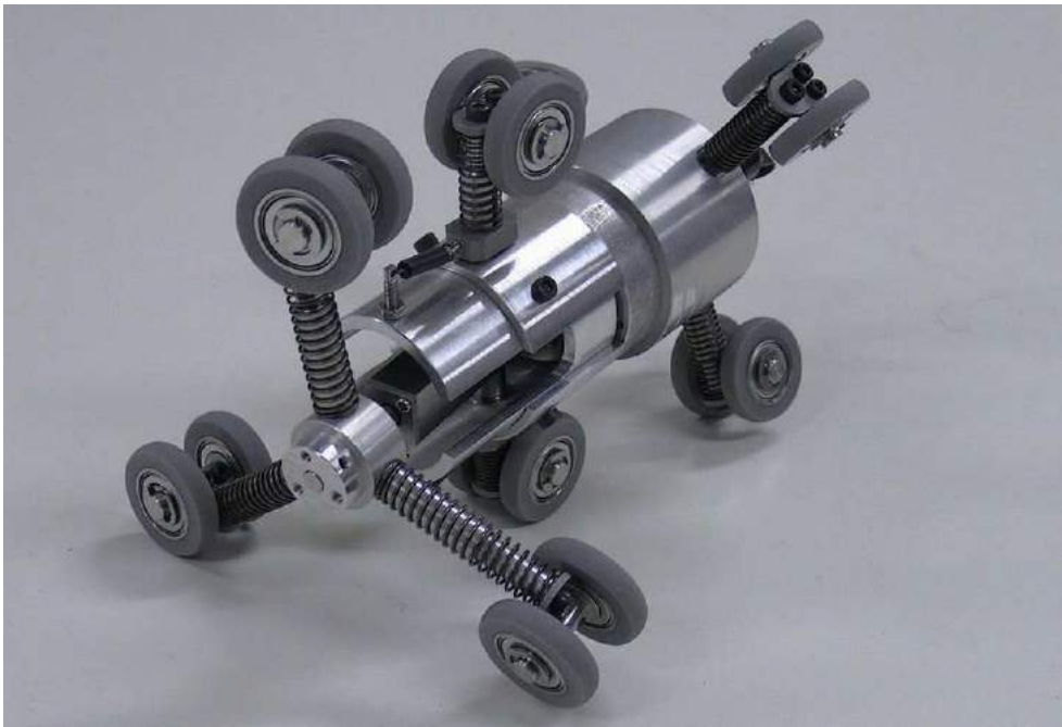
図 4.1: Overview of the screw-driving pipe inspection robot
