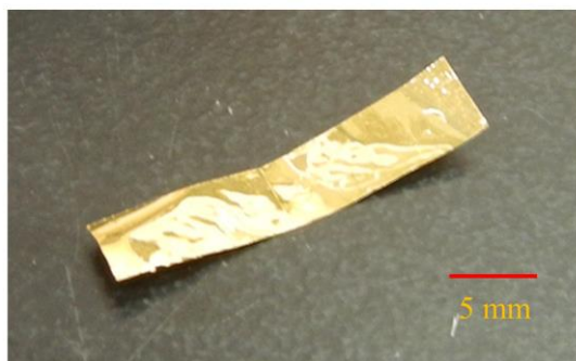
Figure 3.3. Image of the flexible electrode with an Au film on a parylene film substrate.
