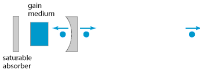
FIGURE 3.13: Schematic setup of a passively mode-locked laser with a saturable absorber mirror [18]
