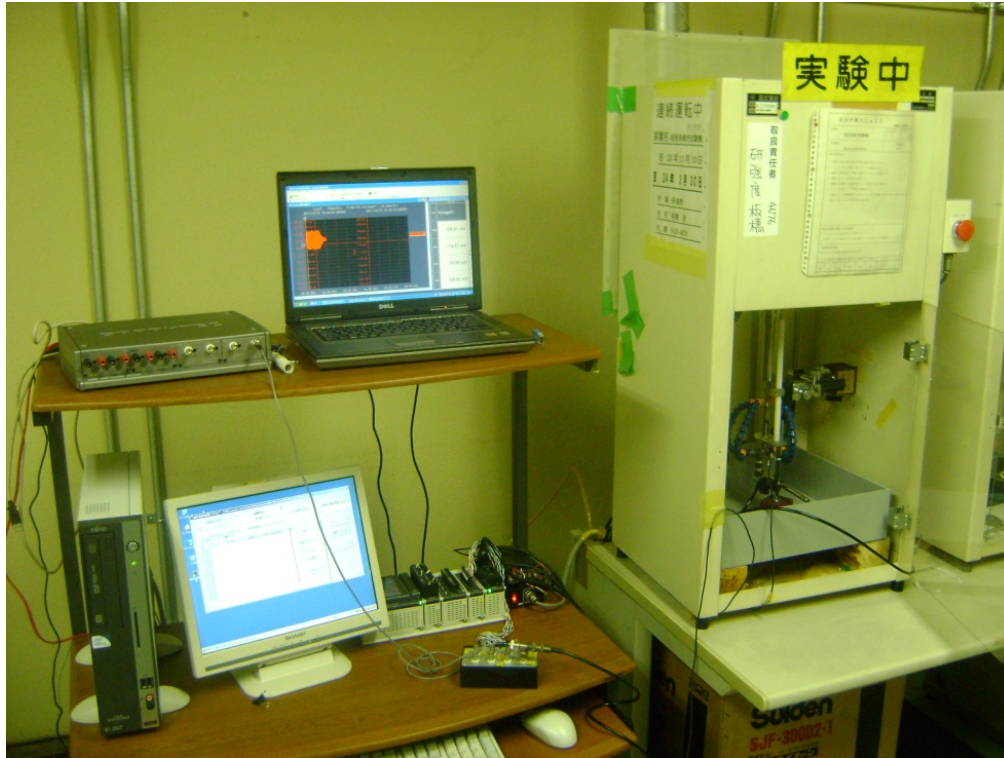
Photo 1 Ultrasonic fatigue testing machine (right) and some control devices (left)
