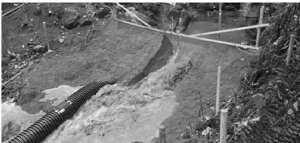
**Photograph 2.1:** Observed results (landslide dam deformation for CASE 1-3).
