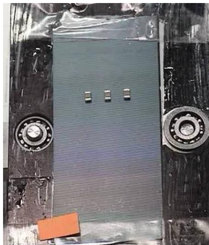
Figure 3.9 Experiment table set up for 2012-capacitors (Mitani et al. , 2007)
