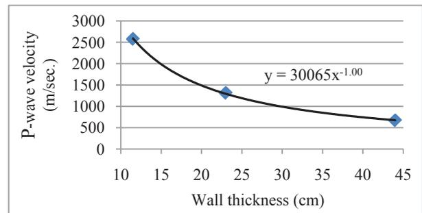
Fig. 4 P-wave velocity with wall thickness
