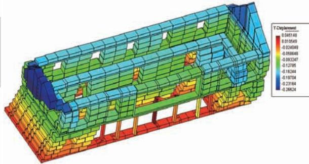
Fig. 10 Deformations in Kobe 1995 earthquake
