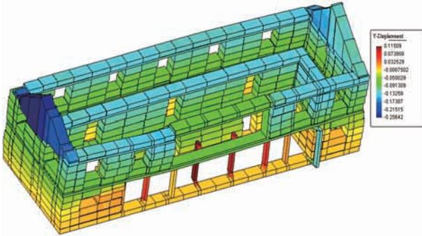
Fig. 9 Deformations in 475 years RP earthquake
