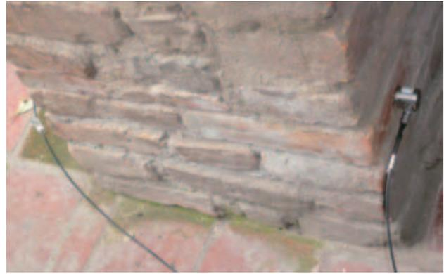
Fig. 3 Instrumentation of two channel Pocket AE
