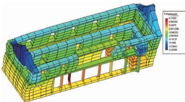
Fig. 12 Deformations in 50% de-amplified El Centro 1940
