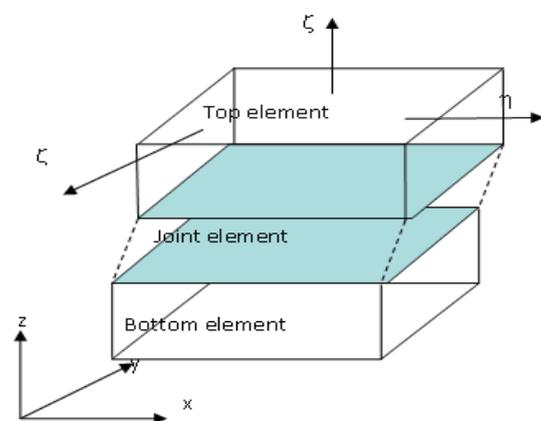
Fig 2 Formulation of solid and joint elements
