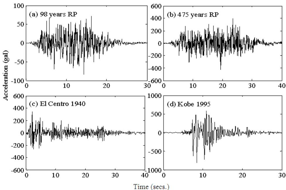
Fig. 8 Input ground motions
