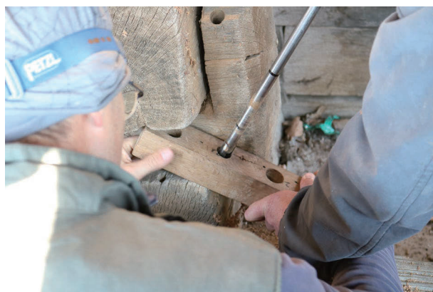
Figure 8 Experts extracting wooden samples during a dendrochronological research at the church from Brusturi, 2018 ©Bogdan Ilieș
