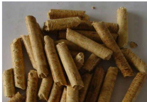
Figure 7: Example: Coconut Husk Pellets (Wandamachine, 2012)
