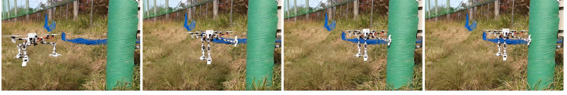
Figure 7.14: Making physical contact with a vertical surface using the manipulator and pushing in the direction of the obstacle using the UAV attitude control.
