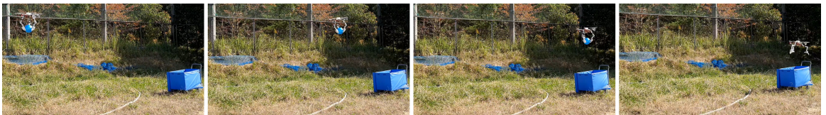
Figure 7.11: Transporting and dropping a spherical object grasped between the manipulators of the UAV into a blue container.
