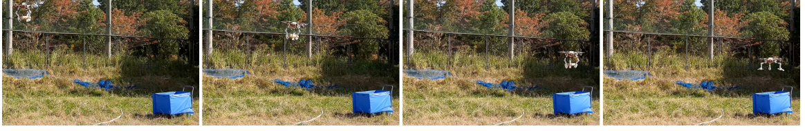
Figure 7.12: Transporting and dropping a cuboid object grasped between the manipulators of the UAV into a blue container.
