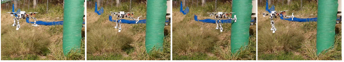
Figure 7.12: Transporting and dropping a cuboid object grasped between the manipulators of the UAV into a blue container.
