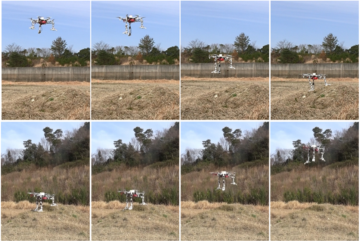
Figure 7.8: Sequential landing process(top) and taking off(bottom) on an uneven surface outdoors. [97]©2019 IEEE.
