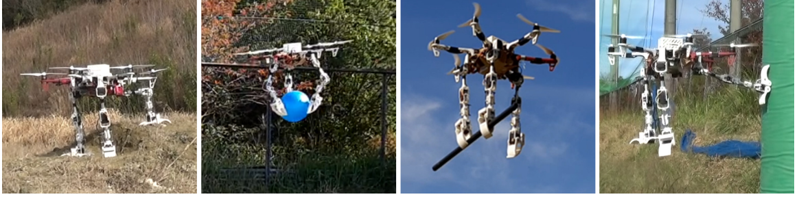
Figure 1.1: Various functions that can be realized with a UAV using a system of three on-board manipulators. From left to right: adaptive landing, transporting large item by means of manipulators, transporting objects by means of grippers, avoiding the UAV body from hitting a vertical surface when flying.
