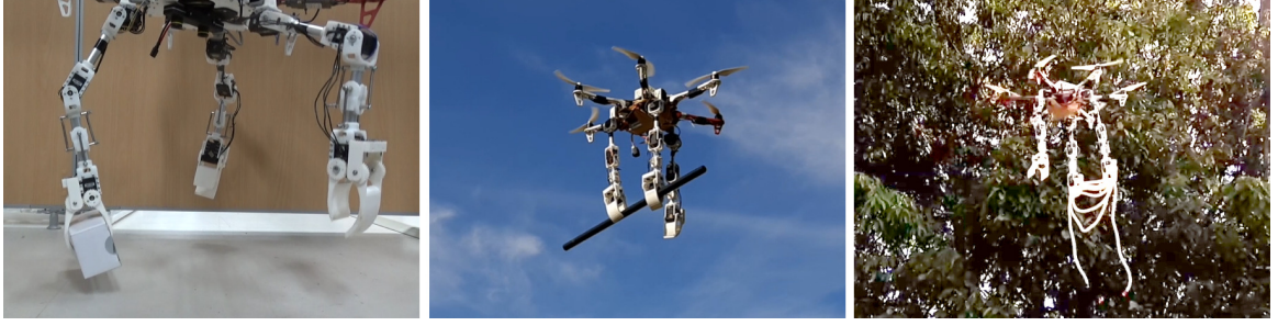
Figure 7.9: Grasping objects using the manipulator’s gripper. (From left to right) Grasping a small cuboid object using single gripper, a long pipe using two grippers and a bundle of rope being carried between two grippers.
