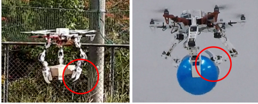
Figure 5.5: Two approaches of grasping a large object using all three manipulators in unison. The gripper is kept open or closed based on the relative distance between the UAV and the object while grasping.
